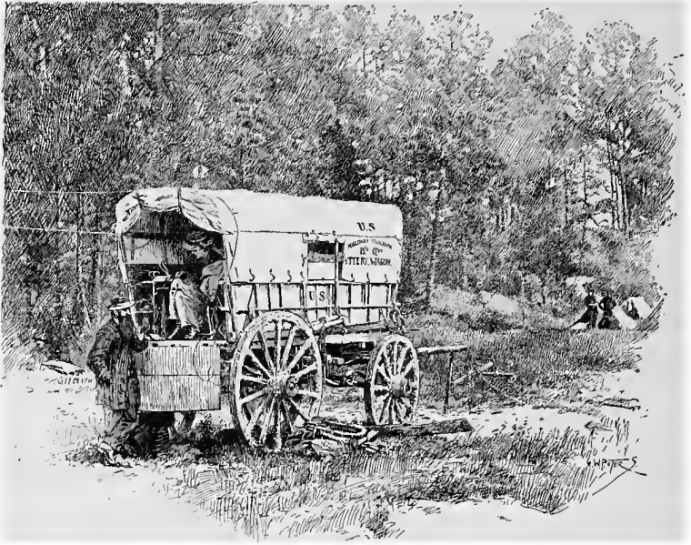
Military Telegraph Battery Wagon at the Headquarters of the Army of the Potomac in front of Petersburg.
